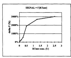
the reaction mixture was diluted 10 times in PBS. 10 µl was transfered to a black microplate followed by 250 µl of SA-XL (5 nM). The measures were performed after 10 min incubation. The graph shows the curve obtained for a serial dilution of Rtase. Quantitation, activity or Rtase inhibitors can therefore be studied using this assay.
